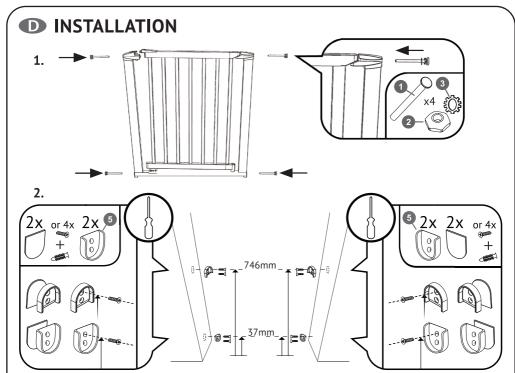
The distances shown above are for screw fixing only. If using adhesive pads, ensure that the wall is clean, dry and free from any grease and align the wall cups to the spindles in the gate. For maximum security, note the opposite orientation of top and bottom wall cups.
