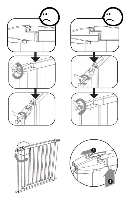
To close the gate, swing the gate door shut from the open position or close it manually by holding the handle and closing the gate door until it locks into position. Always check that the gate is closed and locked before leaving unattended.
